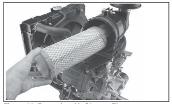
Figure 16. Removing Air Cleaner Element.
